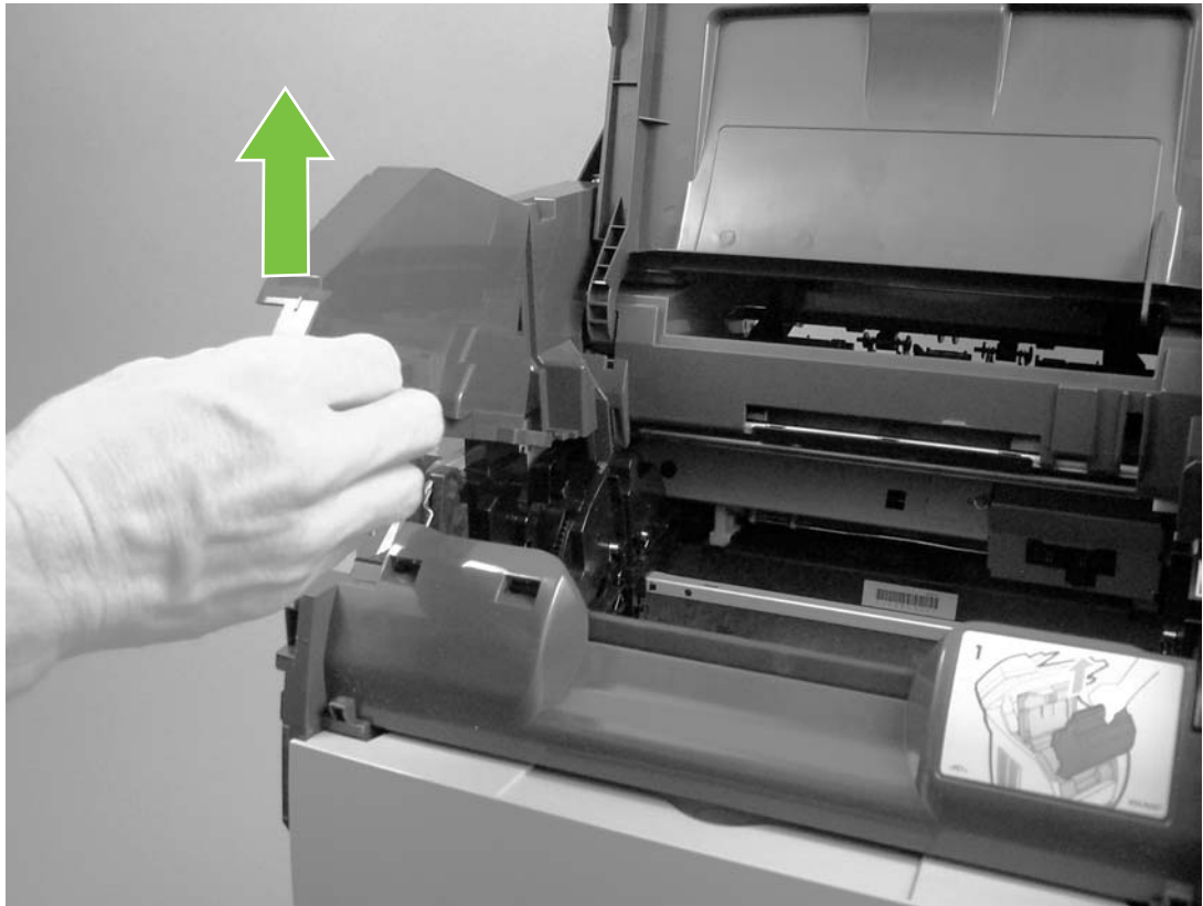
Figure 5-33 Remove the left upper cover (2 of 2)
