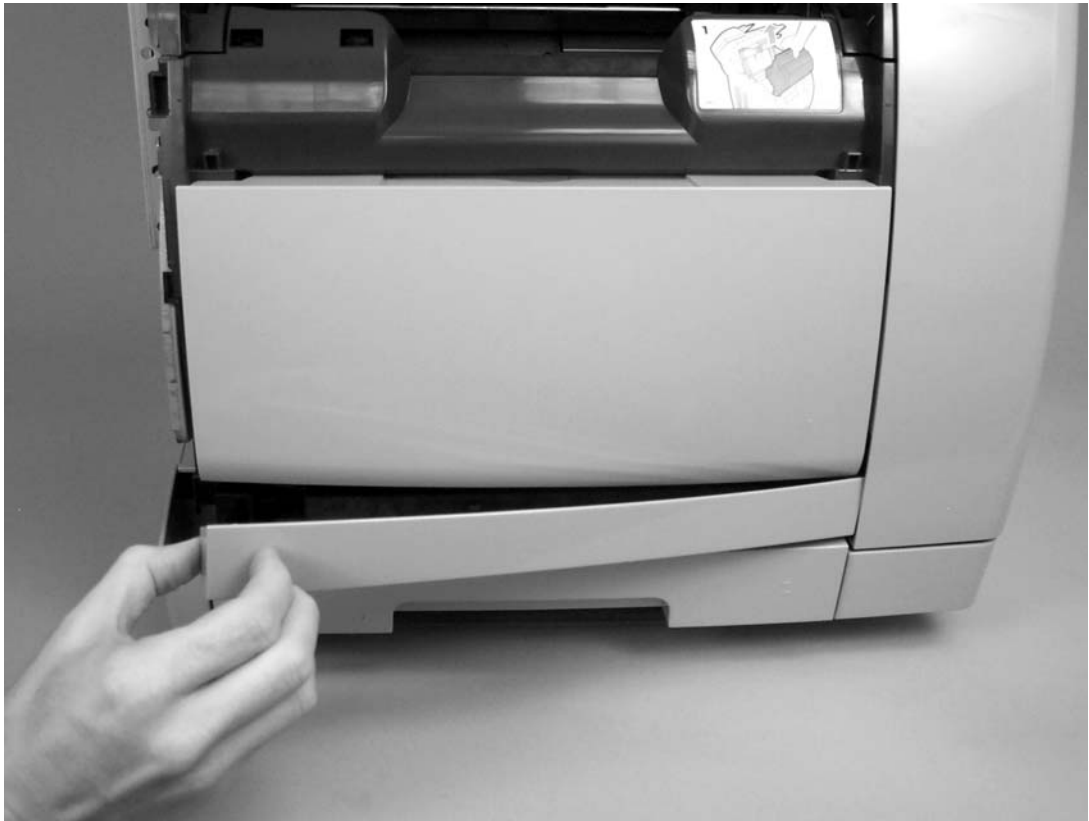
Figure 5-50 Disengage the right-side latch
