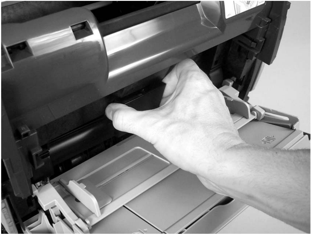
Figure 5-48 Disengage the right-side latch
