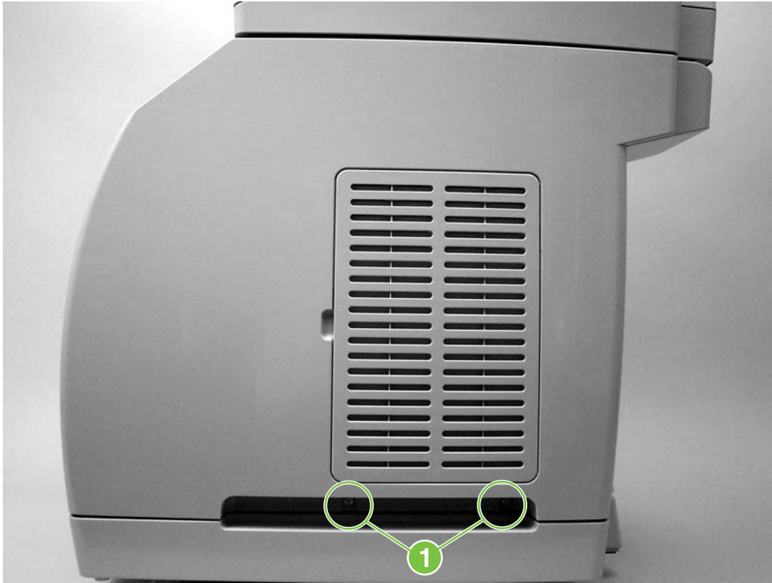
Figure 5-23 Remove the right-side cover (1 of 2)
