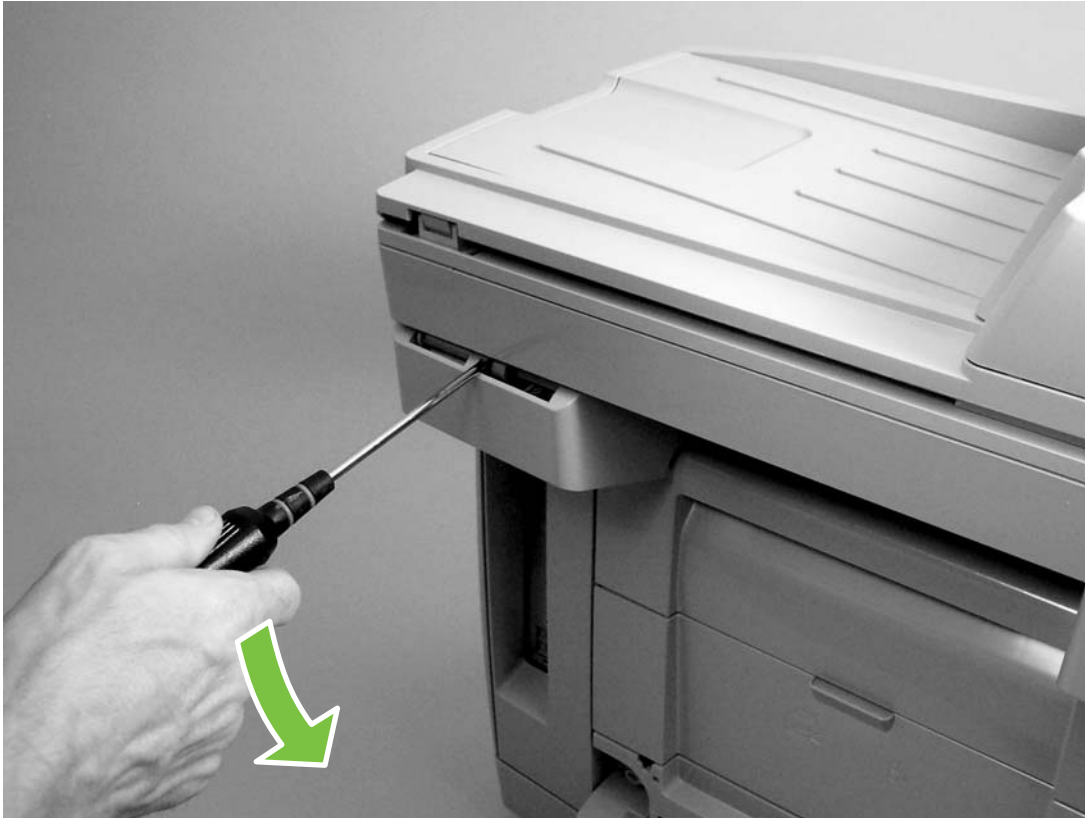
Figure 5-26 Remove the right rear cover (2 of 2)
