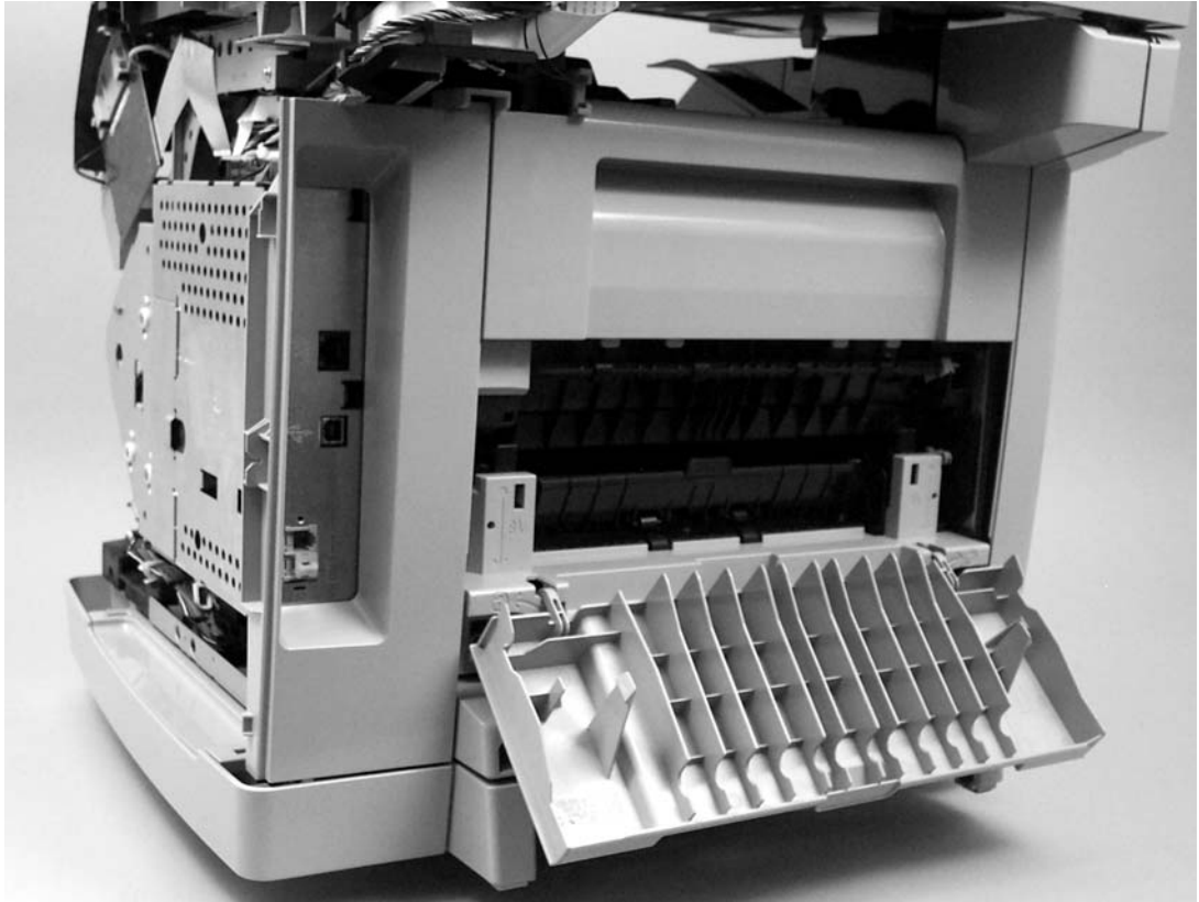
Figure 5-37 Remove the I/O cover (1 of 3)
