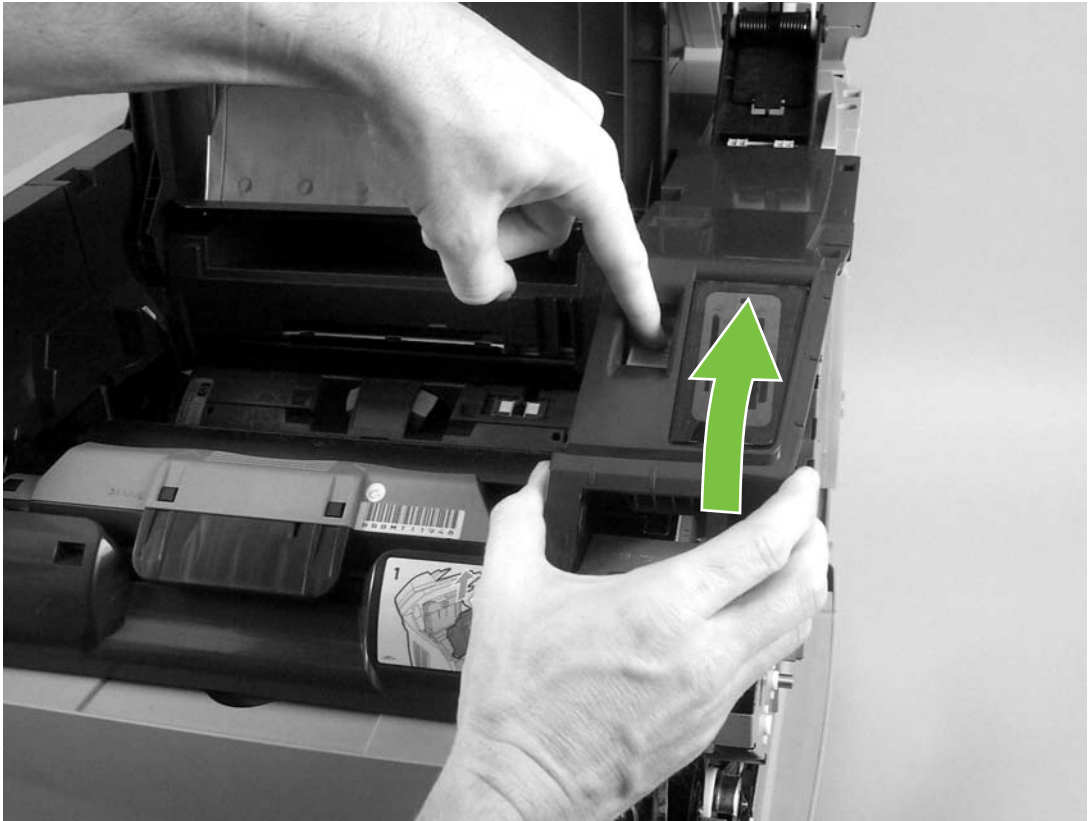
Figure 5-35 Remove the right upper cover (2 of 2)
