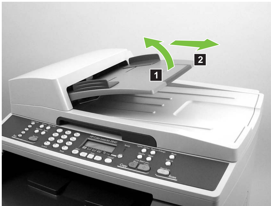
Figure 5-8 Remove the ADF pickup-roller assembly (1 of 5)
