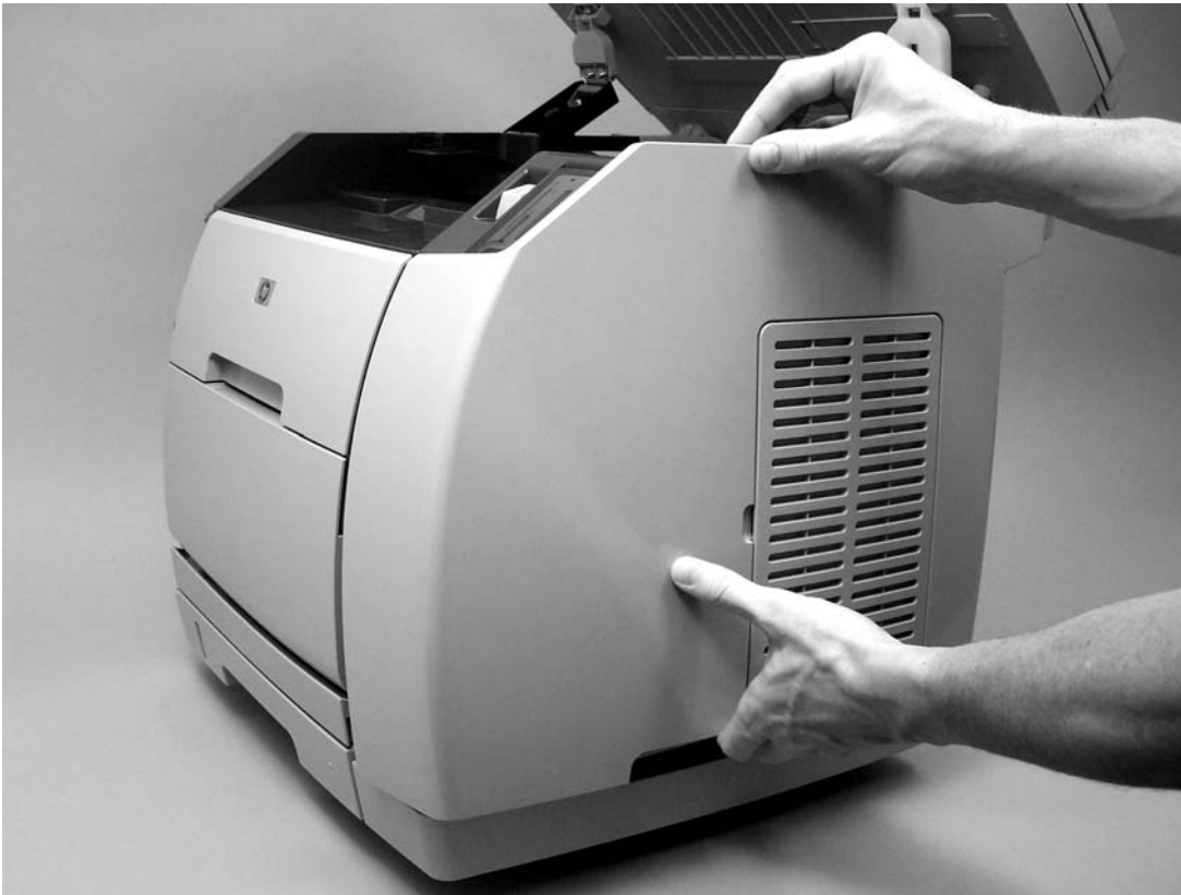
Figure 5-24 Remove the right-side cover (2 of 2)
