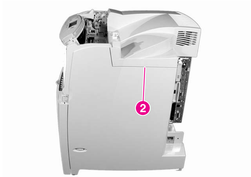
Figure 6-6. Remove the rear top cover (2 of 3)
