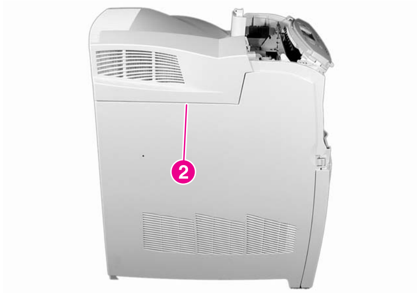
Figure 6-7. Remove the rear top cover (3 of 3)
