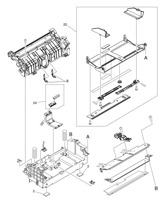
Figure 119. Paper pickup assembly (2 of 2)
