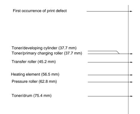
Figure 105. Repetitive image defect ruler
