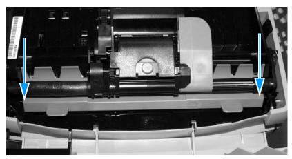
Figure 33. Removing the document feed guide (2 of 2)
