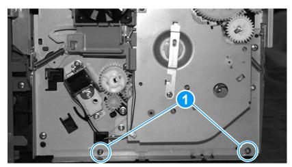
Figure 87. Removing the ECU pan (3 of 5)
