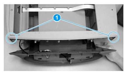
Figure 40. Removing the control panel chassis (2 of 2)
