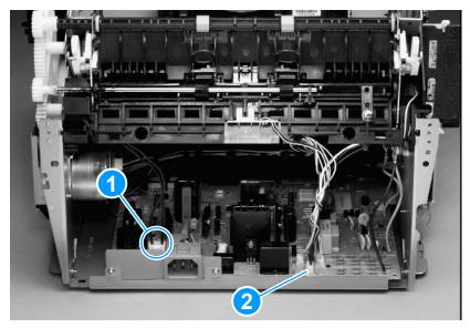
Figure 95. Locating connectors for the heating element check
