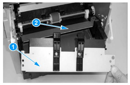
Figure 75. Removing the pickup assembly plate (3 of 3)
