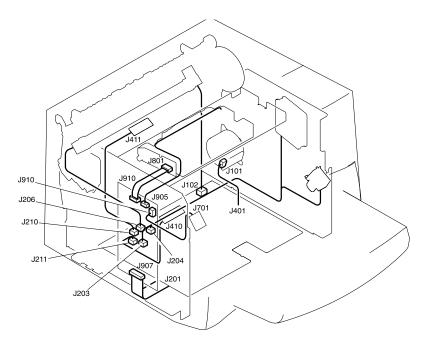
Figure 108. Locations of printer connectors
