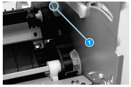
Figure 98. High-voltage connector assembly (right side)
