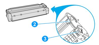
Figure 97. Print cartridge high-voltage connection points (left side)
