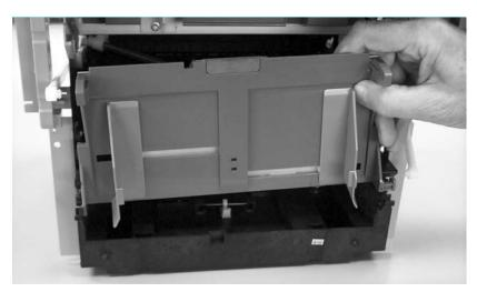
Figure 78. Removing the paper lift-plate assembly (3 of 3)
