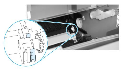
Figure 57. Removing the transfer roller
