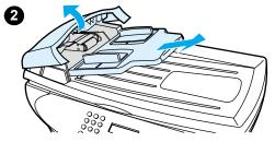
2 Remove the input tray and open the ADF cover.
