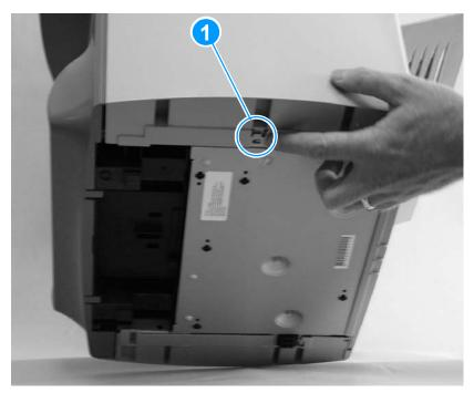
Figure 23. Removing the right side cover (2 of 3)
