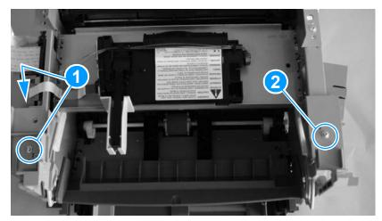
Figure 56. Removing the left and right support covers
