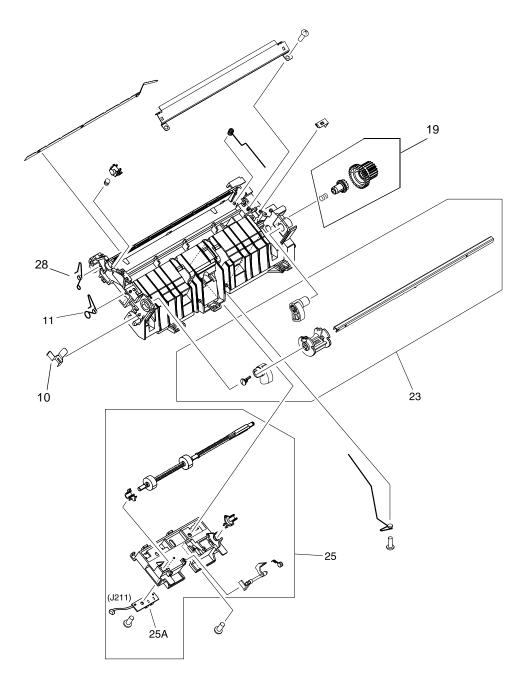
Figure 118. Paper pickup assembly (1 of 2)
