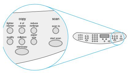
Figure 8. Copy, scan, and start controls
