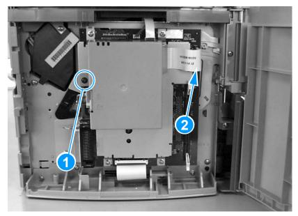
Figure 58. Removing the LIU
