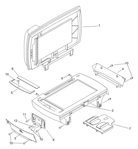
Figure 110. Scanner covers and ADF
