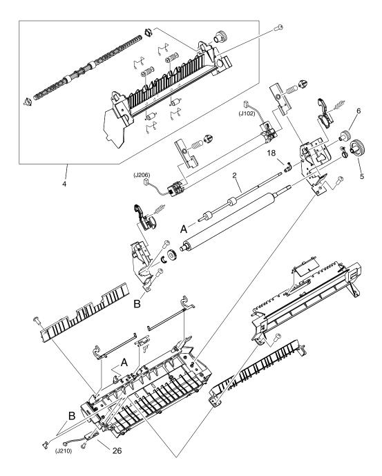
Figure 120. Fuser assembly
