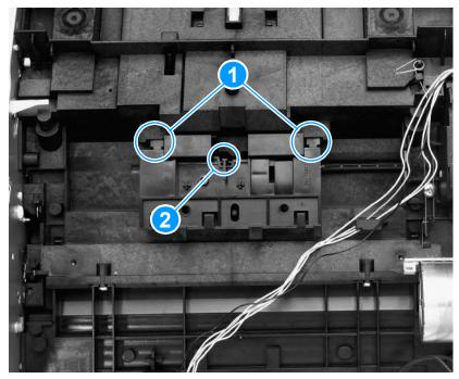
Figure 93. Removing the paper-feed mechanism (4 of 4)
