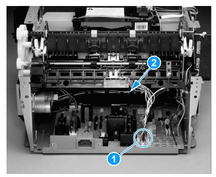
Figure 69.Removing the solenoid (1 of 2)
