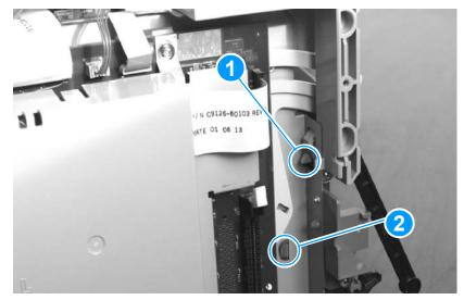
Figure 55. Removing the front guide assembly (3 of 3)
