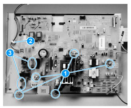
Figure 89. Removing the ECU pan (5 of 5)
