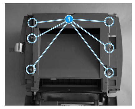
Figure 47. Removing the printer top cover
