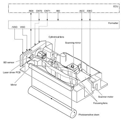
Figure 15. Overview of laser/scanner operation
