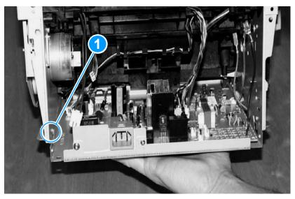
Figure 88. Removing the ECU pan (4 of 5)
