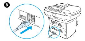
8 Reinstall the input trays, and then plug the product in to turn it back on.
