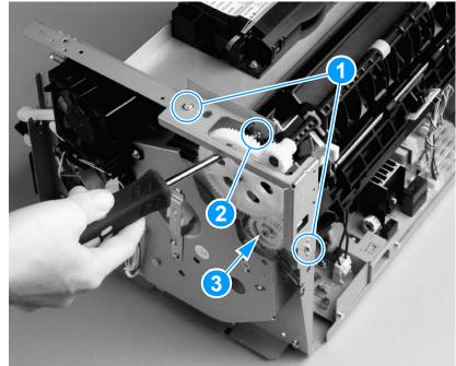
Figure 62. Removing the fuser assembly (1 of 4)
