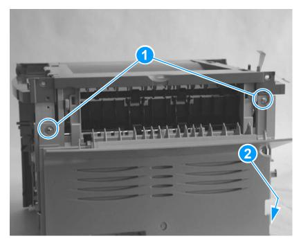
Figure 45. Removing the back cover (1 of 2)
