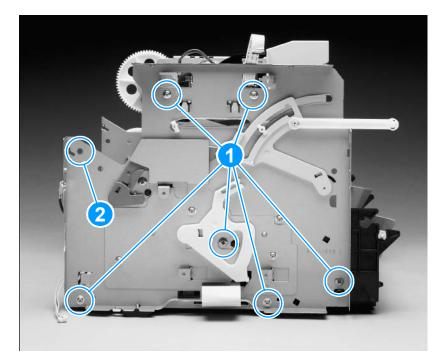
Figure 83. Removing the left plate assembly
