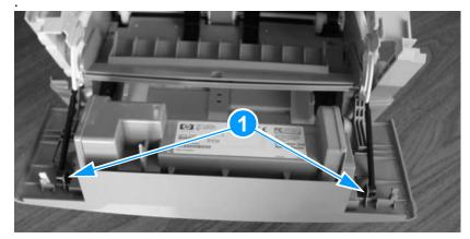
Figure 48. Removing the print cartridge door (1 of 2)
