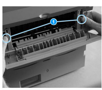
4 Press down and hold the two release levers (callout 1) and pull off the back cover.
