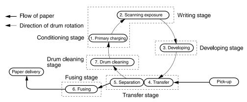
Figure 17. Image formation block diagram
