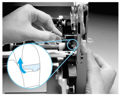
Figure 81. Removing the right plate assembly (1 of 2)
