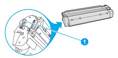
Figure 96. Print cartridge high-voltage connection points (right side)
