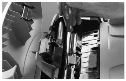
Figure 34. Removing the ADF separation pad
