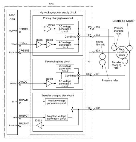
Figure 16. High-voltage power supply circuit
