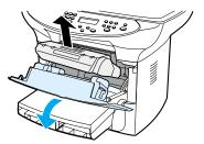
Figure 21. Removing the print cartridge
