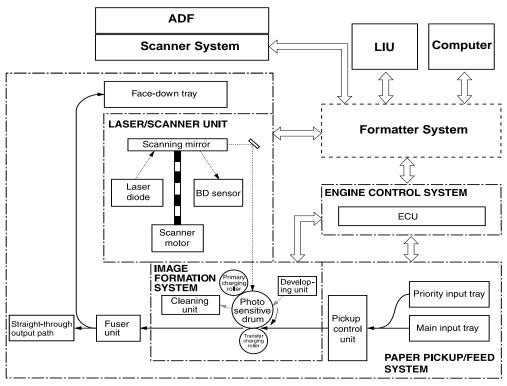
Figure 13. Printer unit functional block diagram
