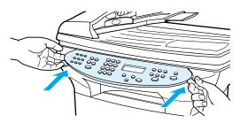
Figure 35. Removing the control panel bezel
