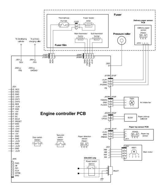
Figure 107.Main wiring (2 of 2)
