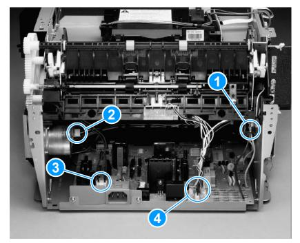
Figure 85. Removing the ECU pan (1 of 5)
