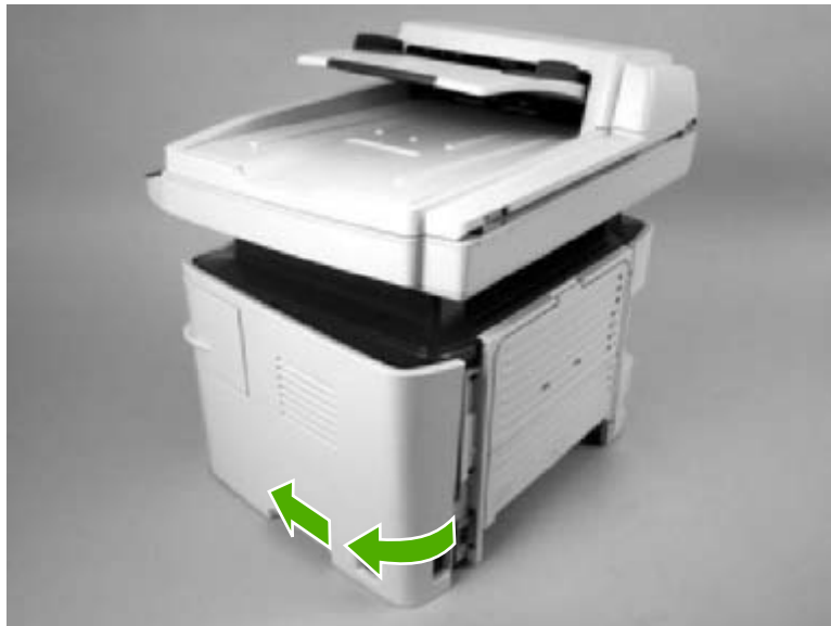
Figure 5-8 Remove the right cover (4 of 4)
