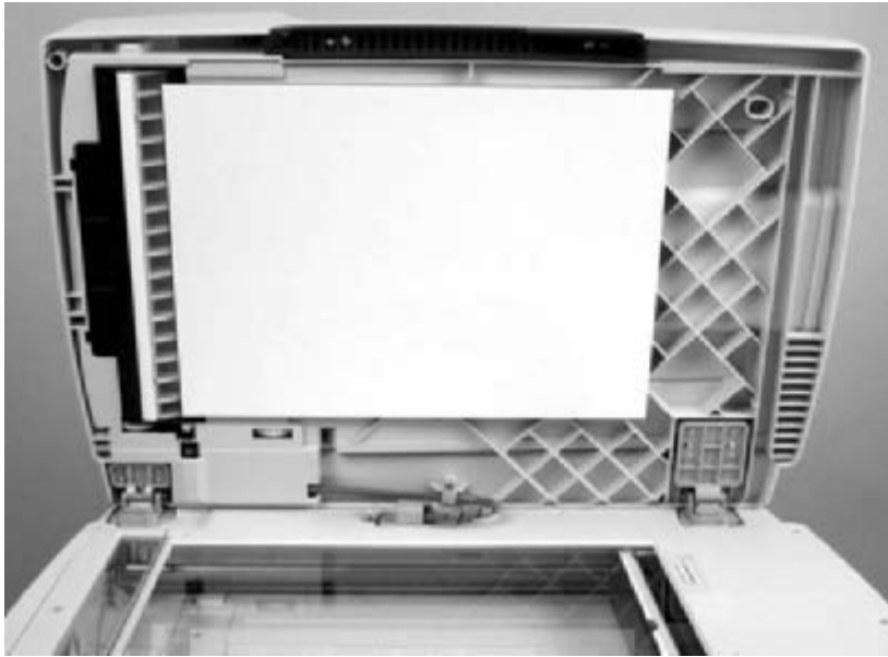
Figure 5-25 Remove the ADF assembly (1 of 3)
