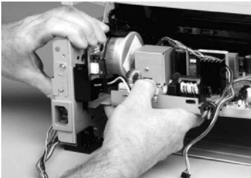
Figure 5-77 Remove the ECU (6 of 8)
