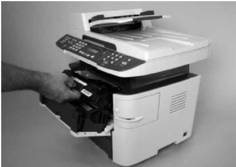
Figure 5-4 Remove the print cartridge (2 of 2)
