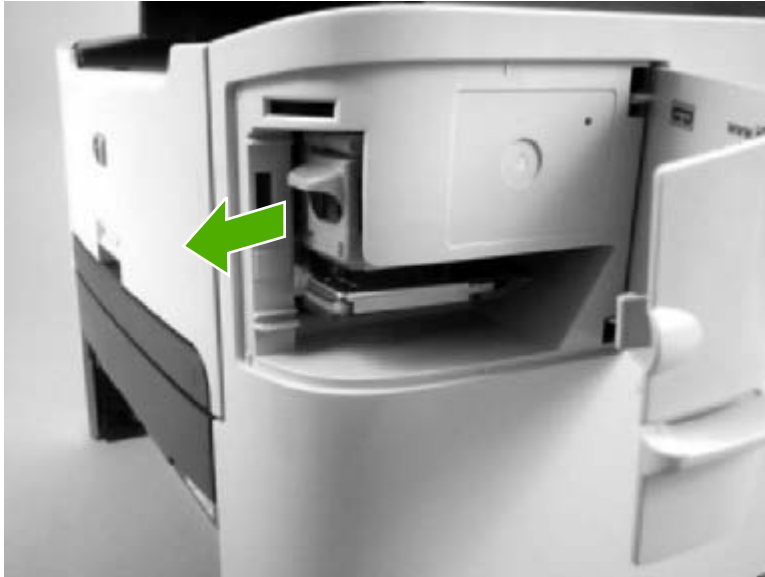
Figure 5-5 Remove the right cover (1 of 4)
