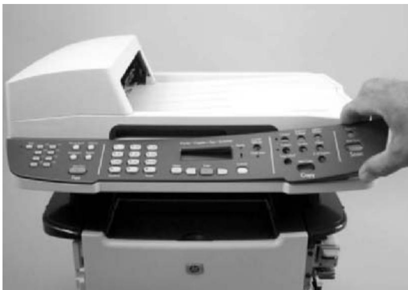
Figure 5-31 Remove the bezel and control panel (1 of 4)
