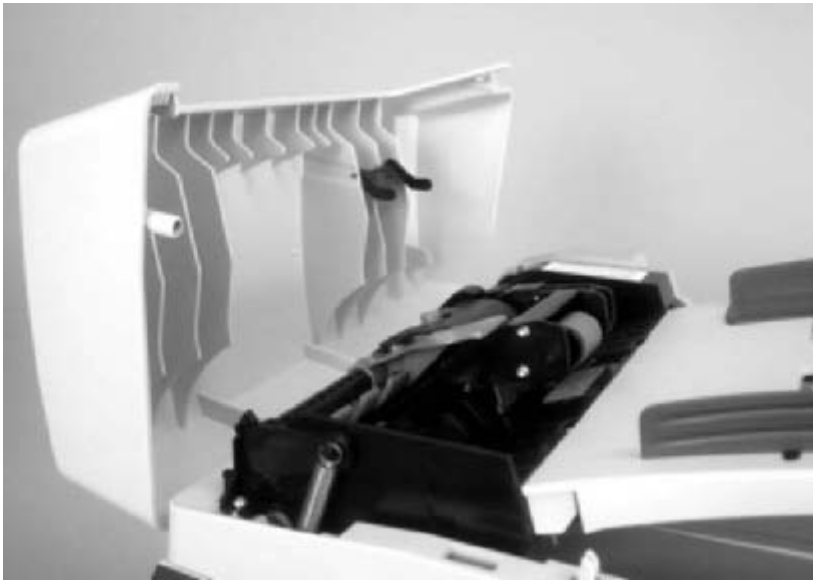
Figure 5-19 Replacing the ADF pickup-roller assembly (1 of 6)
