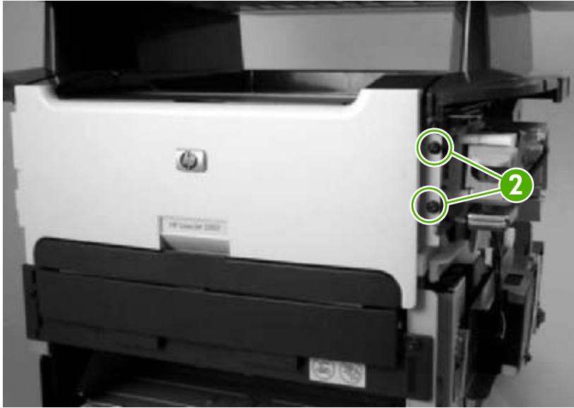
Figure 5-36 Remove the convenience-stapler assembly (2 of 2)
