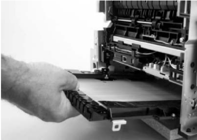
Figure 5-50 Remove the duplex assembly (3 of 3)
