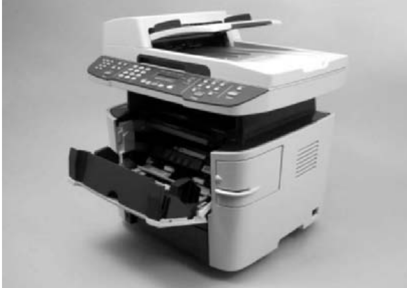
Figure 5-3 Remove the print cartridge (1 of 2)
