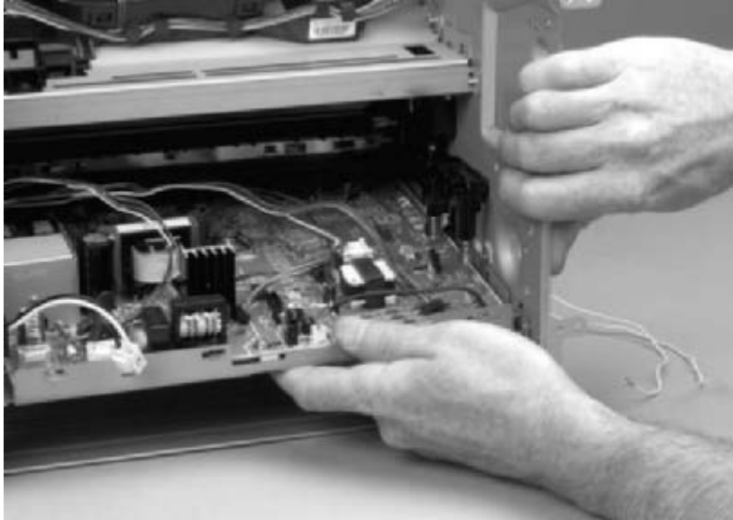
Figure 5-78 Remove the ECU (7 of 8)
