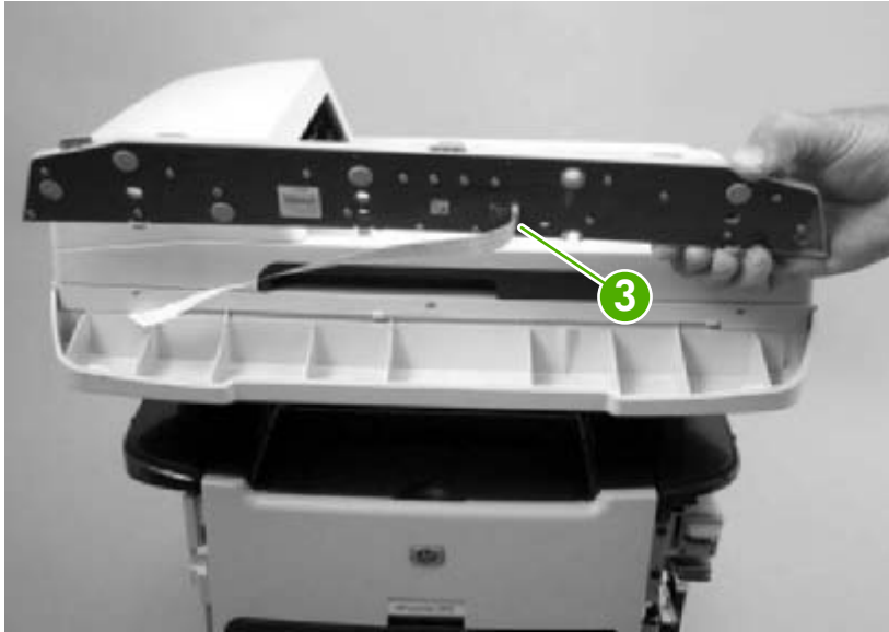
Figure 5-34 Remove the bezel and control panel (4 of 4)
