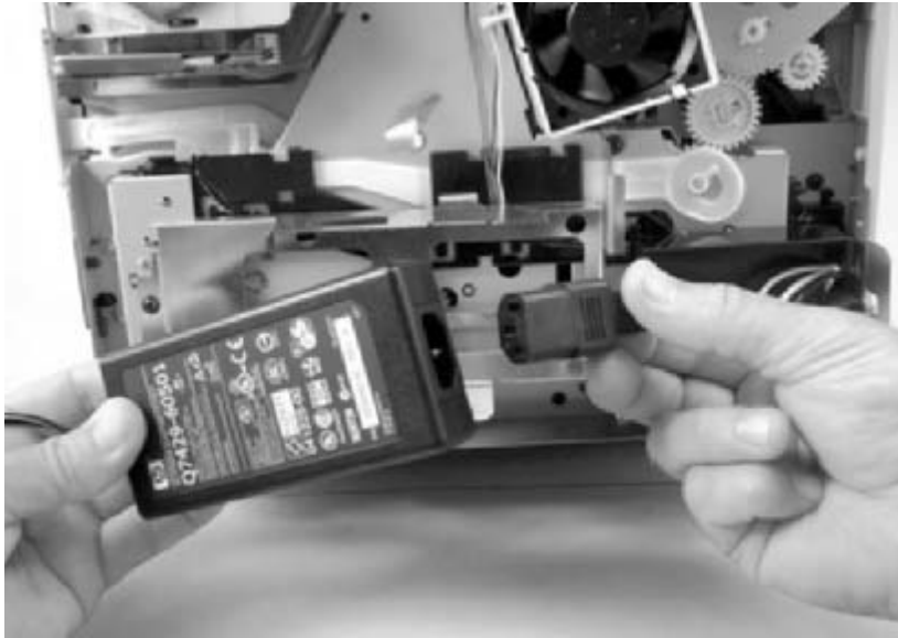
Figure 5-39 Remove the convenience-stapler power assembly (3 of 3)
