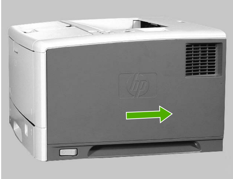
Figure 5-39 Removing the right cover
