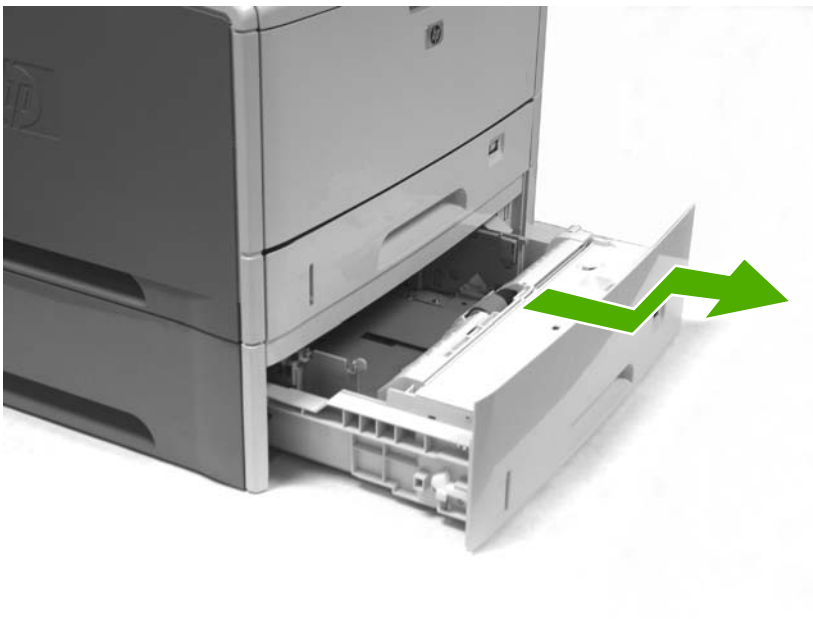
Figure 5-11 Removing the tray 3 retard roller (1 of 2)
