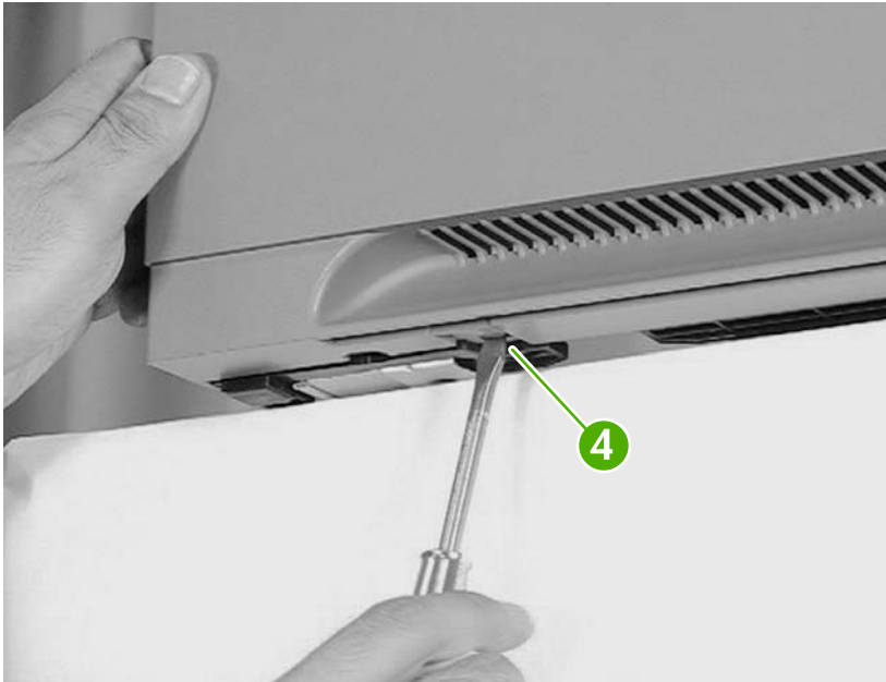
Figure 5-53 Removing the left cover (4 of 5)
