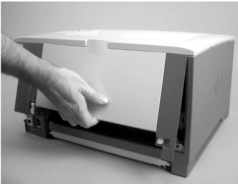
Figure 5-44 Removing the face-up bin (4 of 4)
