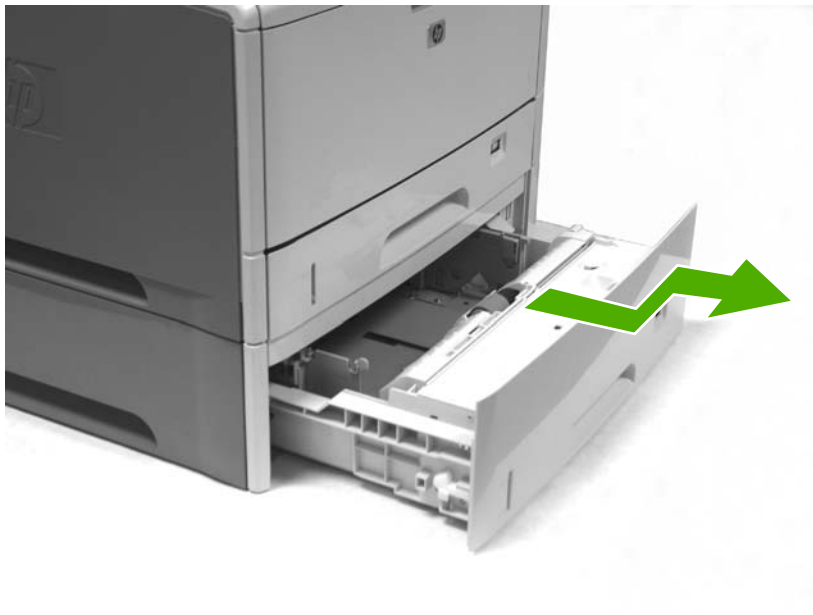
Figure 5-13 Removing the tray 3 pickup and feed rollers (1 of 2)
