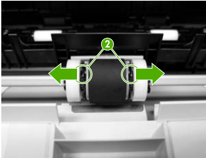
Figure 5-4 Removing the tray 1 pickup roller (2 of 3)
