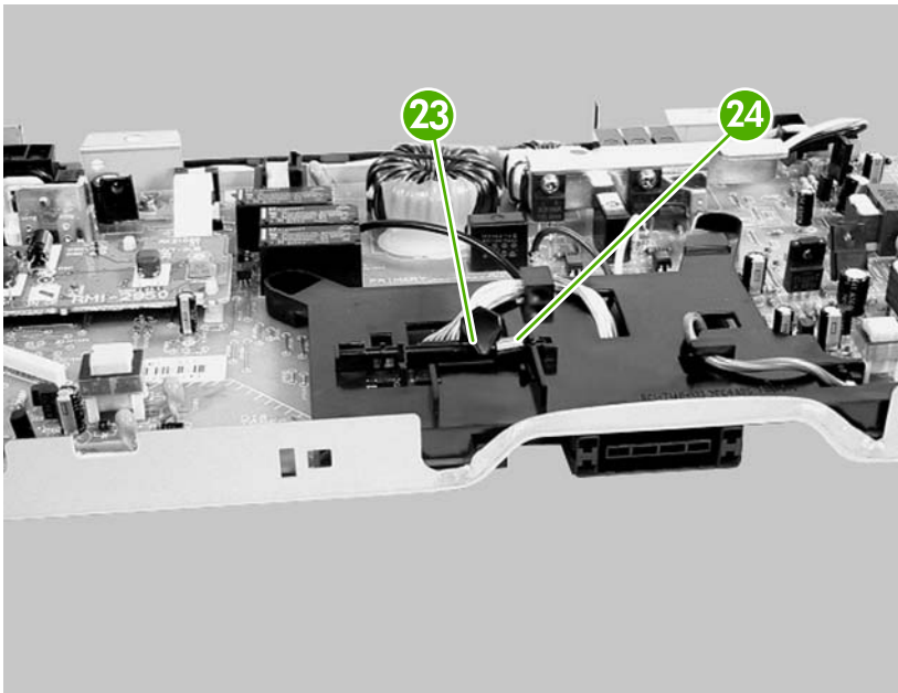
Figure 5-147 Removing the high-voltage power supply (16 of 17)
