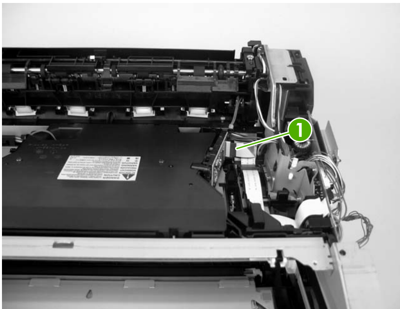
Figure 5-80 Removing the laser/scanner (1 of 3)
